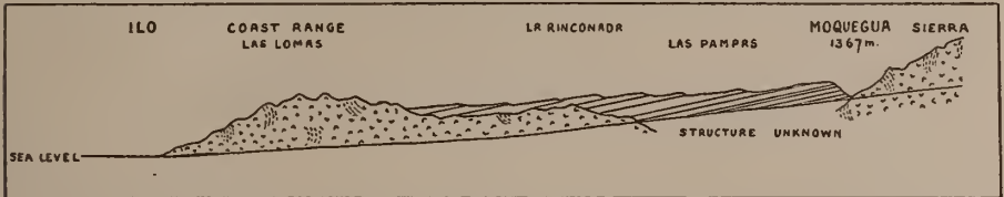
FIG. 172—Geologic relations of Coast Range, desert deposits, and Maritime Cordillera at Moquegua, Peru. After G. I. Adams; Bol. de Minas del Perú, Vol. 2, No. 4, 1906, p. 20.
